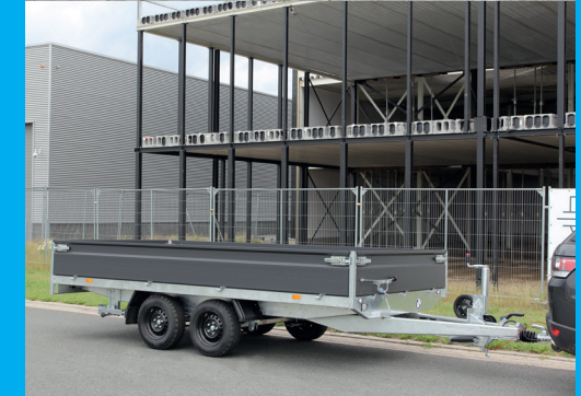
Standard: 90° swivelling heavy duty prop stands incl. support crank not mounted.
